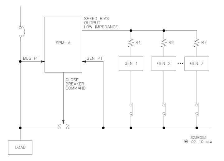
Figure 3-2. Synchronizing Bus to Bus
